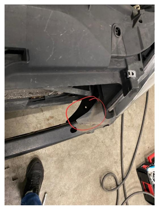
3. Remove some of the material on the inside of the strut shown.
