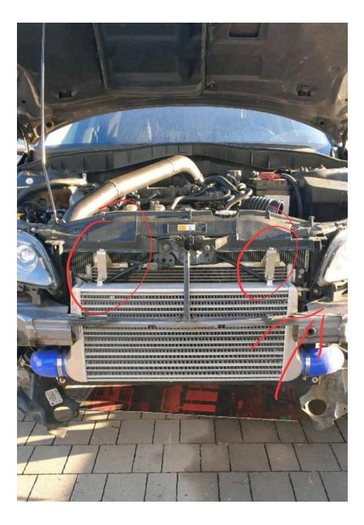
7. After the intercooler has been attached, you can now start with the intercooler piping.
