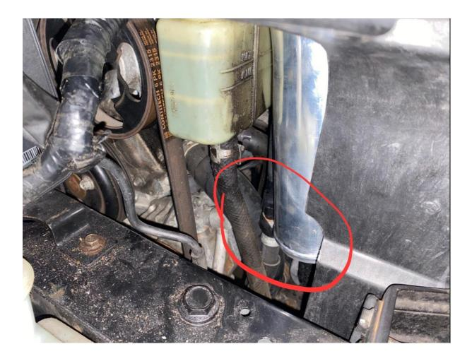
11. On the cold side where the piping goes to the intake manifold, a hole must be cut through the plastic shield of the water cooler. Please also note that you do not swap the two pipes (see photo)
