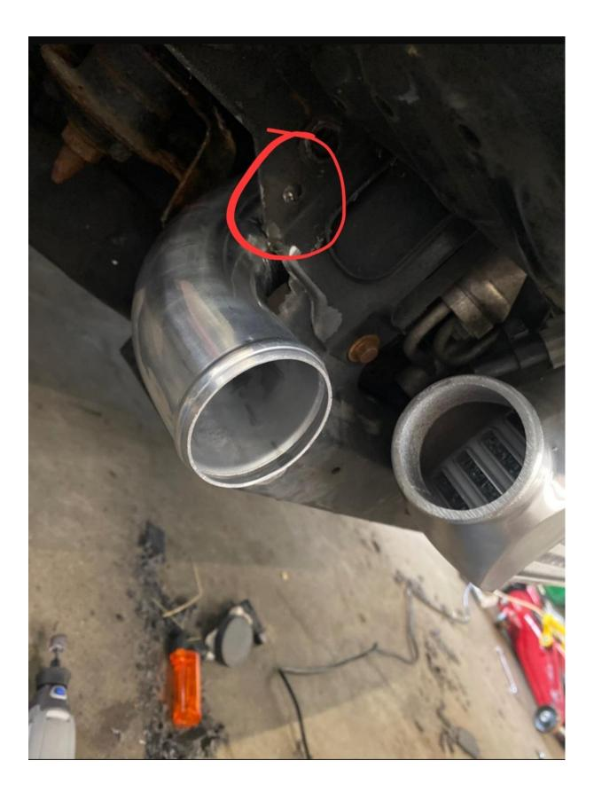
10. The position of the long pipe that goes to the turbocharger is shown here. To make it easier to attach and fasten the silicone connector, remove the headlight (passenger side)
