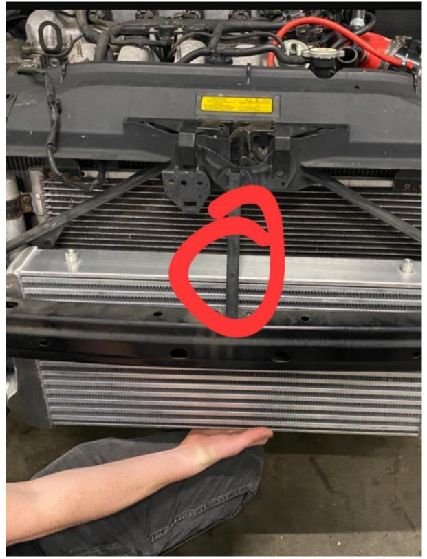
4. The exact height of the intercooler is determined by the holder supplied.
